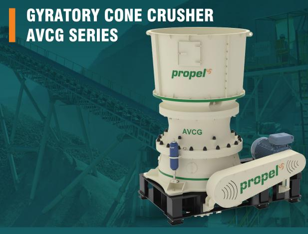
The Gyratory Cone Crusher delivers increased capacity with reduced maintenance and downtime. It guarantees trouble-free operation in varying feed conditions with a high reduction ratio. It has large and stable feed opening, steep cavity and effective strokes.
