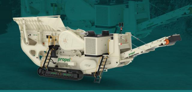
The elevated mouth opening of the TMJ Series single toggle Jaw Crushers ensure significant production saving by eliminating frequent bridging of stone in feed opening. Optimum jaw nip angle reduces laminar product shape, ensures even manganese wear-off with increasing production.
